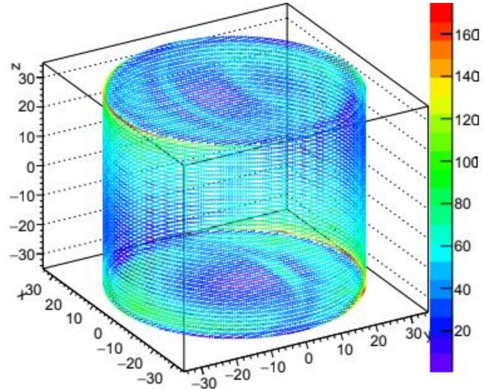
➤ Difficulty in compensating for the geomagnetic field at the top and bottom of walls
