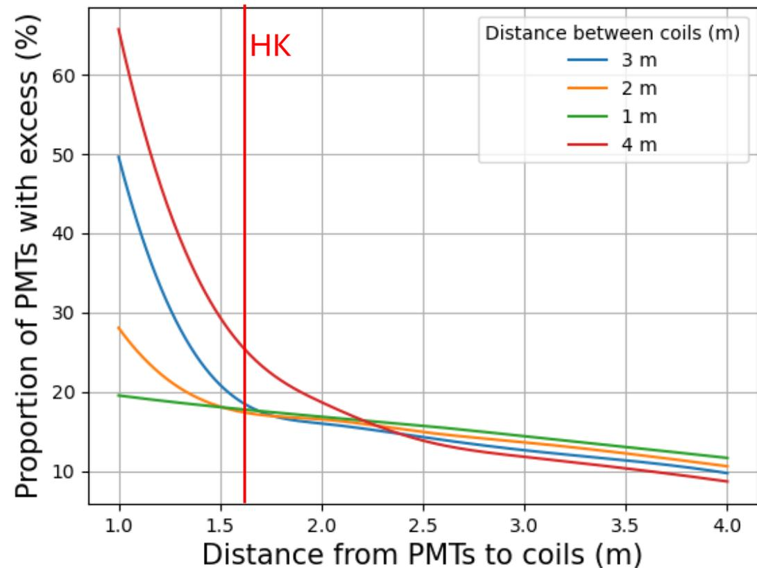
Distance from PMTs to coils in HK = 1.6 m
