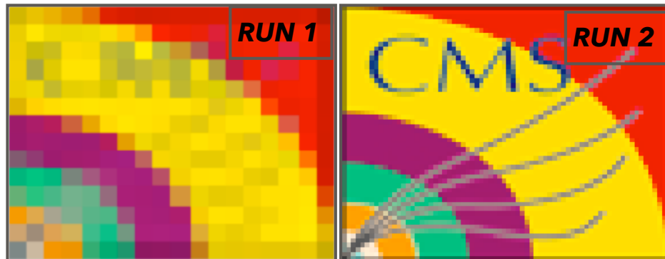
Phase-1 Upgrade: increased calorimeter granularity LHC Run-1 2009 - 2012 LHC Run-2 2015 - 2018
